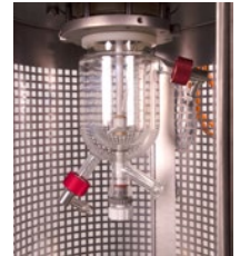
Glass vessel with Pt100-sensor and stirrer.
