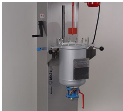
Tilttable reactor for easy cleaning and maintenance
