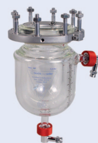
Type 1I Glass vessel with heating jacket and vacuum insulation jacket, without drain valve 0.5 / 1.0 / 1.6 l max. 12 bar / 200°C
