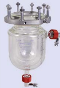
Type 1I Glass vessel with heating jacket and vacuum insulation jacket, without drain valve 0.5 / 1.0 / 1.6 / 2.0 l max. 12 bar / 200°C
