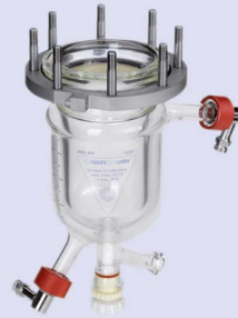
Type 1B Glass vessel with heating jacket and drain valve 0.25 / 0.5 / 1.0 / 1.6 / 2.0 l max. 6 bar / 200°C
