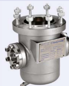
Type 4 Metal vessel with heating jacket, 2 sight glasses and drain valve 1.0 / 1.5 / 2.0 / 3.0 / 5.0 l max. 60 bar / 250°C
