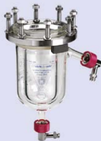
Type 1 Glass vessel with heating jacket, without drain valve 0.25 / 0.5 / 1.0 / 1.6 / 2.0 l max. 12 bar / 200°C
