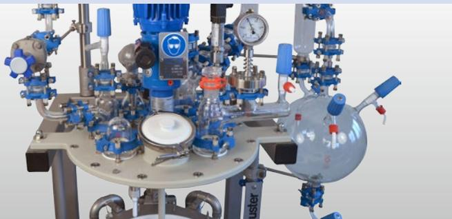
Solid steel cover plate, PFA coated, 7 ports
