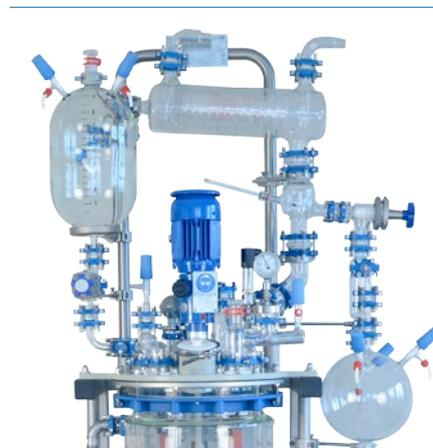
Glass overhead with spiral condenser, reflux divider, phase separator and distillate receiver
