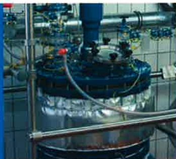
Reactor with removable insulation 取り外し可能な断熱付反応容器
