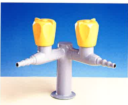
6303 TWO WAY TAP AT 90°, FIXED NOZZLE OUTLET, PUSH-TURN GAS HEADWORK
